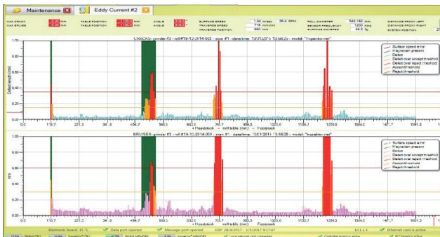
► Pomini Inspektor System EC 2D screen shot
