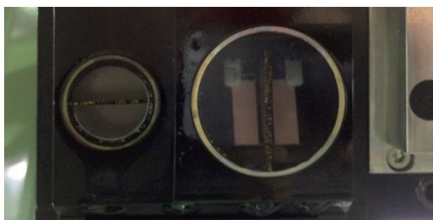
► Left Side is the US (0°) degree probe while on right side the Ultrasound Creeping Wave
