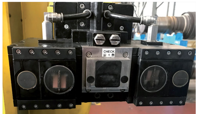
► Close-up of typical Inspektor Head with probes
